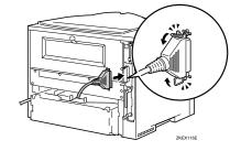
Securely attach the other end of the parallel cable to your computer's parallel port. Secure the cable
